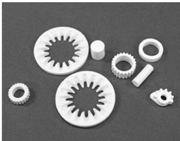
Fig. 7. Illustration of the ultimate alumina ceramic parts fabricated by using HEMA system.
